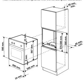
In order to ensure adequate ventilation, the back panel of the cabinet unit must be removed. Installing the oven so that it rests on two strips of wood is preferable. If the oven rests on a continuous, flat surface, there must be an aperture of at least  $45 \times 560$  mm.
